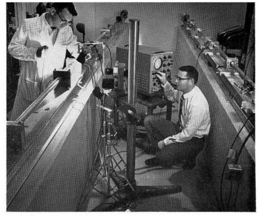
HIGH STRAIN RATE TEST of a plastic material is prepared by E. R. Dunaway (left) and O. L. Burchett on the Hopkinson pressure bar device. High speed photographic coverage will yield a visual record plus superimposed oscilloscope data on the film. Test will show the strain rate sensitivity and the failure mode of the material.
